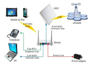
To obtain the best radio signal level and connection quality, the user can rotate the CPE slowly in horizon direction to find the best signal direction, then fixed it with the anchor ear. The CPE radio signal strength level can be observed from the RF LEDs mounted on the lower panel as shown below. The more LEDs on, the better the signal strength.
