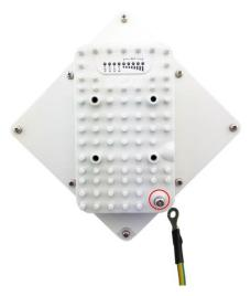
Connect one of a grounding cable to the grounding screw and firmly tighten the grounding screw. Connect the opposite end of the grounding cable to a good ground(earth) connection.
